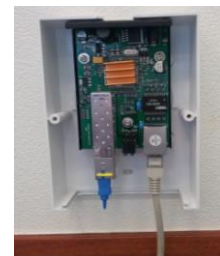
Wall-mount Fiber-to-Home Optical Node (ONU-Mini_1)
