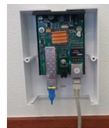
Wall-mount Fiber-to-Home Optical Node (ONU-Mini_1)
